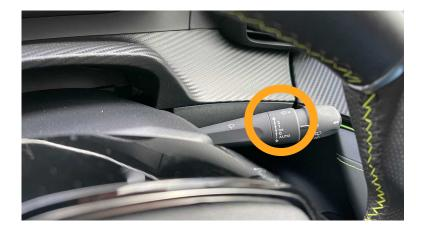
Pull the lever towards the steering wheel and hold while the screen wash is sprayed onto the windscreen.
