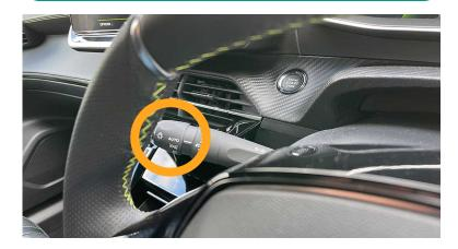
Twist the end of the lever all the way until you see the dipped headlight warning light illuminates on the dashboard
